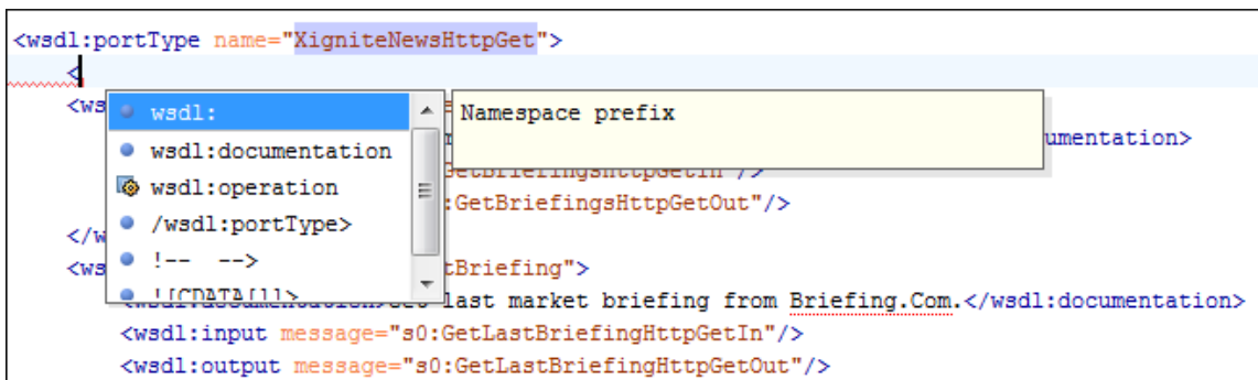
Figure 265. Namespace Prefixes in the Content Completion Assistant
